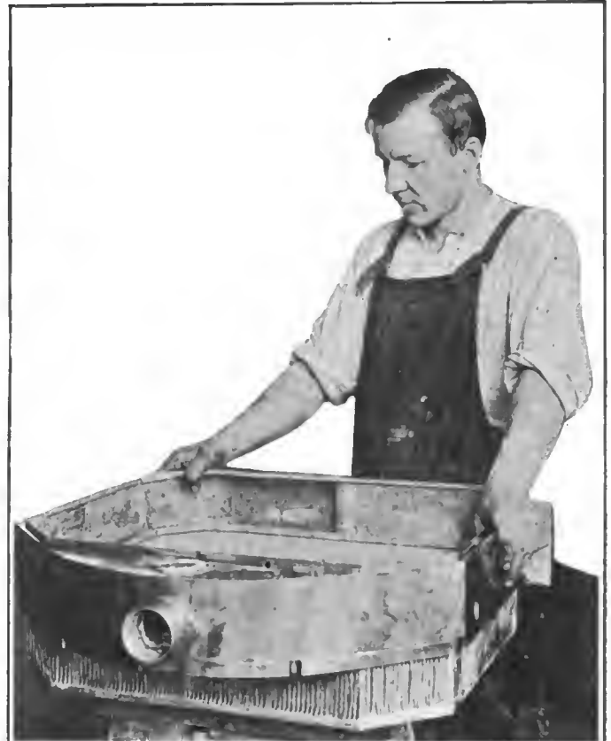
Stage 10—Giving the final test for leaks in the finished radiator
